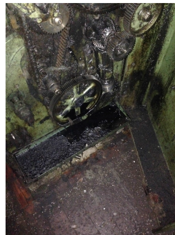
Photo 10 – Oil staining observed on textile machinery
